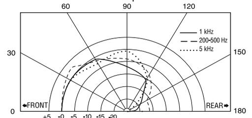
Fig. 3 Horizontal-Plane Polar Response
